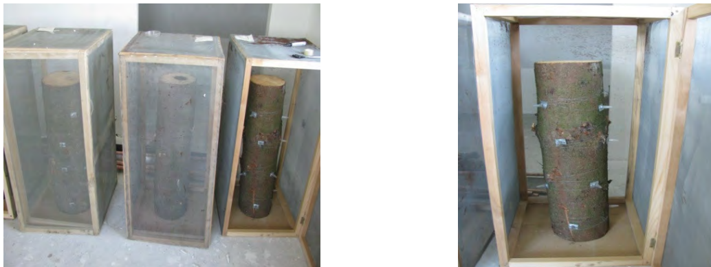
FIGURE 1. EXPERIMENTAL CAGES USED IN LABORATORY B. bassiana BIOASSAYS
